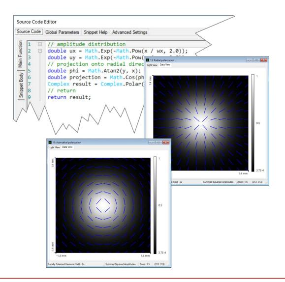
Polarization is one of the most characteristics properties of light, with much beyond the basic concept of global polarization, where light can only be linearly, circularly or elliptically polarized. We present here how to create in VirtualLab a radially and an azimuthally polarized source, illustrating in the process the programming of light sources and the potential of the Combined Light Source feature.
